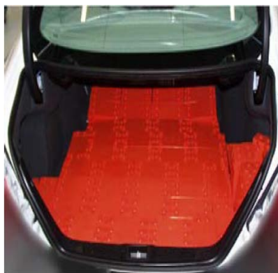
Figure 1. Trunk capacity calculation by DIN70020 standard [7].
